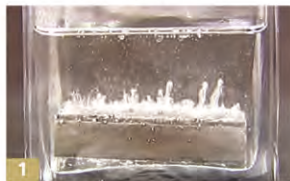
FIGURE 1. HYDROGEN ESCAPING FROM A WELDMENT.
