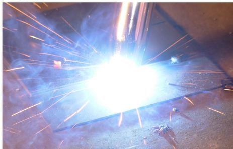
An alternative is to use MIG Braze process, using a copper silicon alloy wire SIFMIG 968 (CuSi3). SIFMIG 968 has a relatively low melting point approx 980 C.
