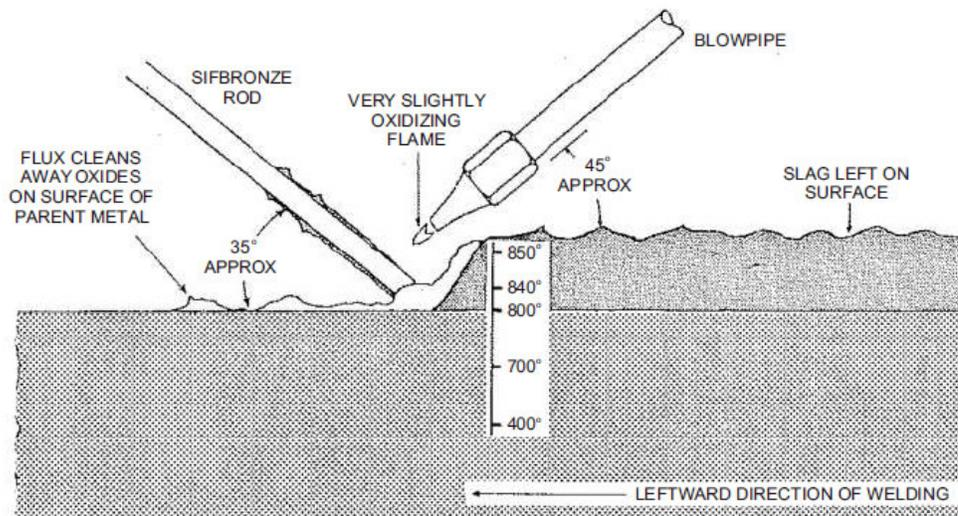
Sifbronzing is an almost universally recognised way of describing the low temperature bronze welding of sheet steel, cast iron and other metals. The reason behind this fact summarises why Sifbronze, the company which first developed and promoted the technique, is generally considered to be a supplier of top-quality welding rods, wires, fluxes and equipment.
