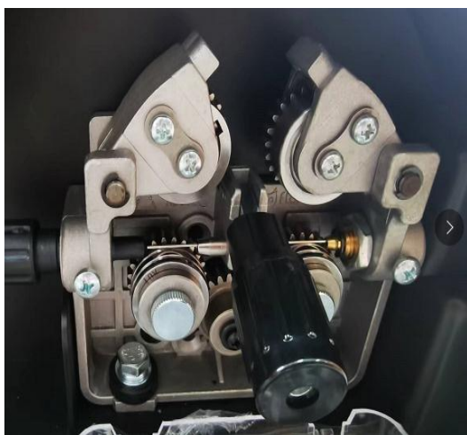
Arrange the wire feed wheel of corresponding wire diameter
