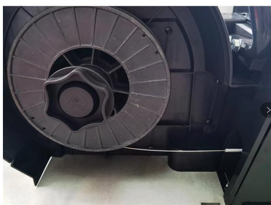
Pay attention to the wire feed direction, cross the wire into the wire feed pipe
