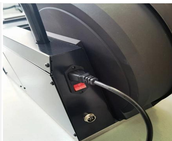
Insert the attached power wire into the 3-pin type socket.
