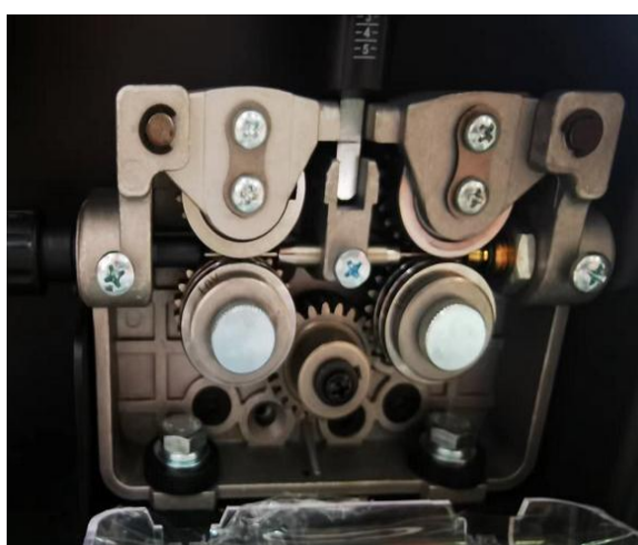
Press the wire feed wheel with pressing handle, then loosen it properly
