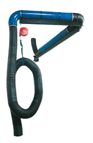
The Fumex balancing block solution, type ASA without pivoting arm, is equipped with hose, balancing block and suspension belt. The extractor is mounted hanging from the ceiling or other high location. For wall mounting, wall bracket ASA V is available.
