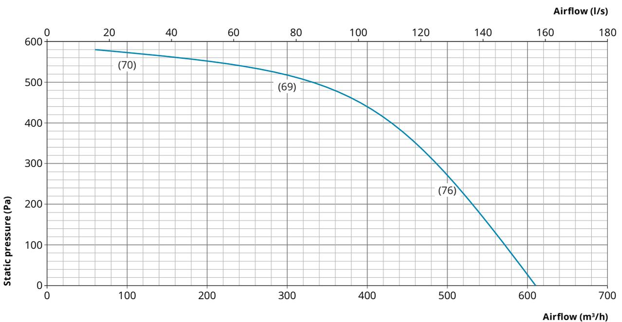
Ambient fan noise, as measured 1 metre from fan dB(A).
